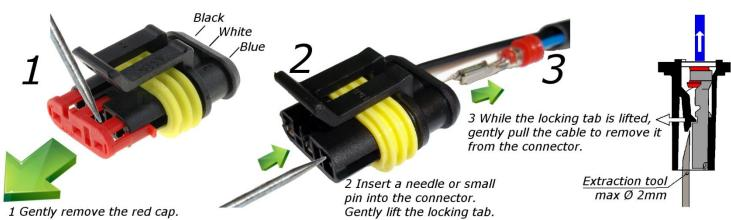
To reassemble the plug, insert the terminals back in place till the locking tab clicks in and put back the red cap.
