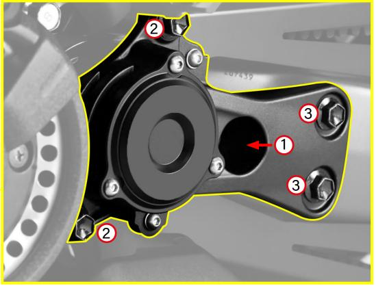
Remove the original pinion from the support using the appropriate extraction tool.
